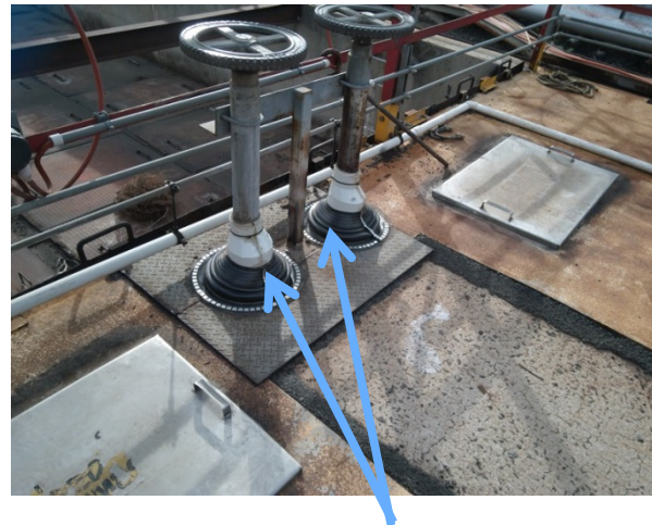
Gaps around handwheel penetrations sealed
