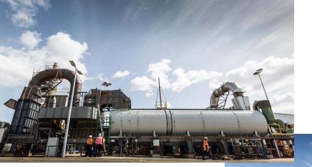
The new oxidiser takes advantage of improved thermal performance of a refractory lining
